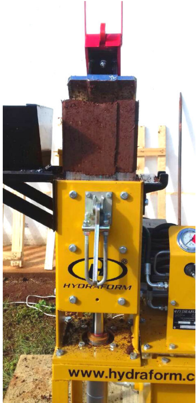
Ndlangamandla & Dlamini load mud into the Hydraform brick maker.
