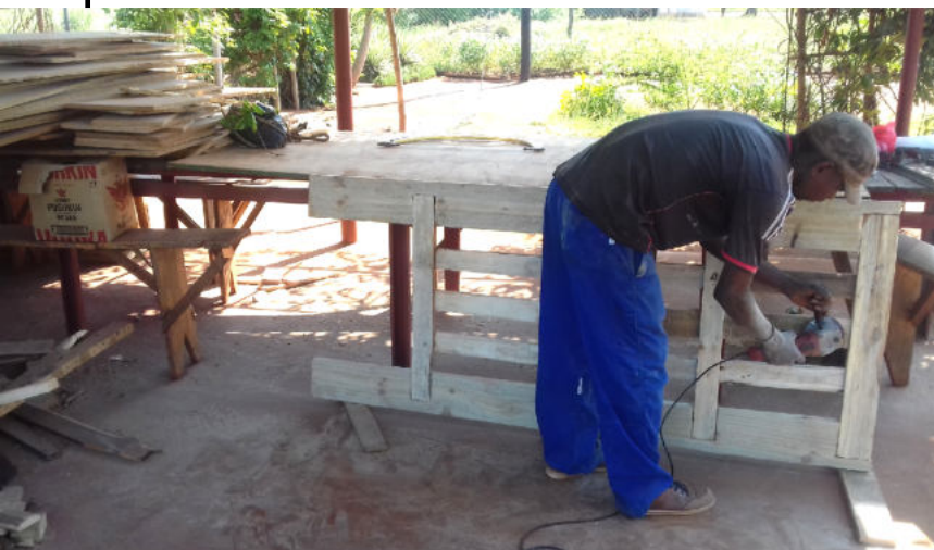
Bunk beds, tables, seats and shelves were made from reclaimed wooden pallets.
