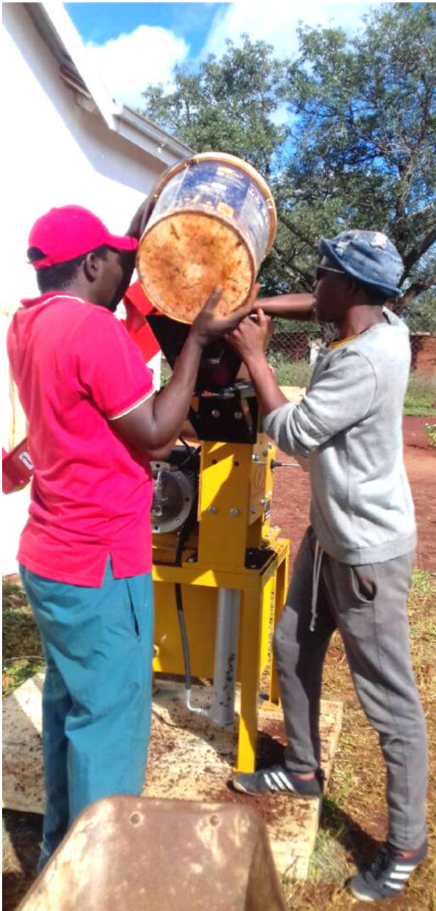
Ndlangamandla & Dlamini load mud into the Hydraform brick maker.
