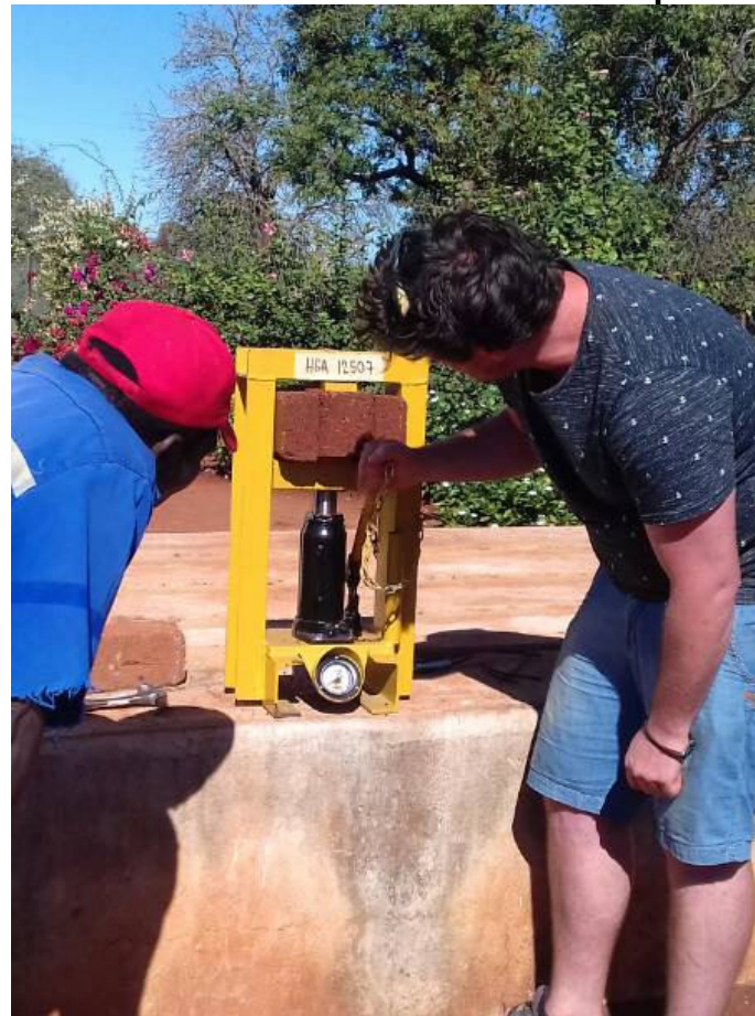
Ndlangamandla & Wolmarans pressure testing the strength of the mud bricks.
